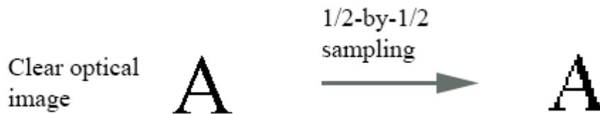
Figure 3 Simulation of binning causing aliasing. (Note: for best quality, view at 100% ratio.)
