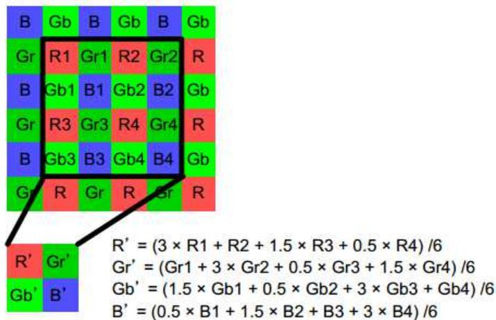
Figure 2 Sensor read out schemes for normal frame rate (4K 30fps) and high frame rate (1080p 60/96fps), showing the binning technique does not change the physical size of the area read out, thus keeping the field of view. Only the pixels at the two corners of the active region are shown.
