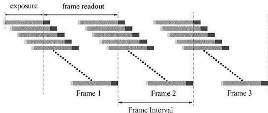
Figure 4 Timing of the sensor exposure.
