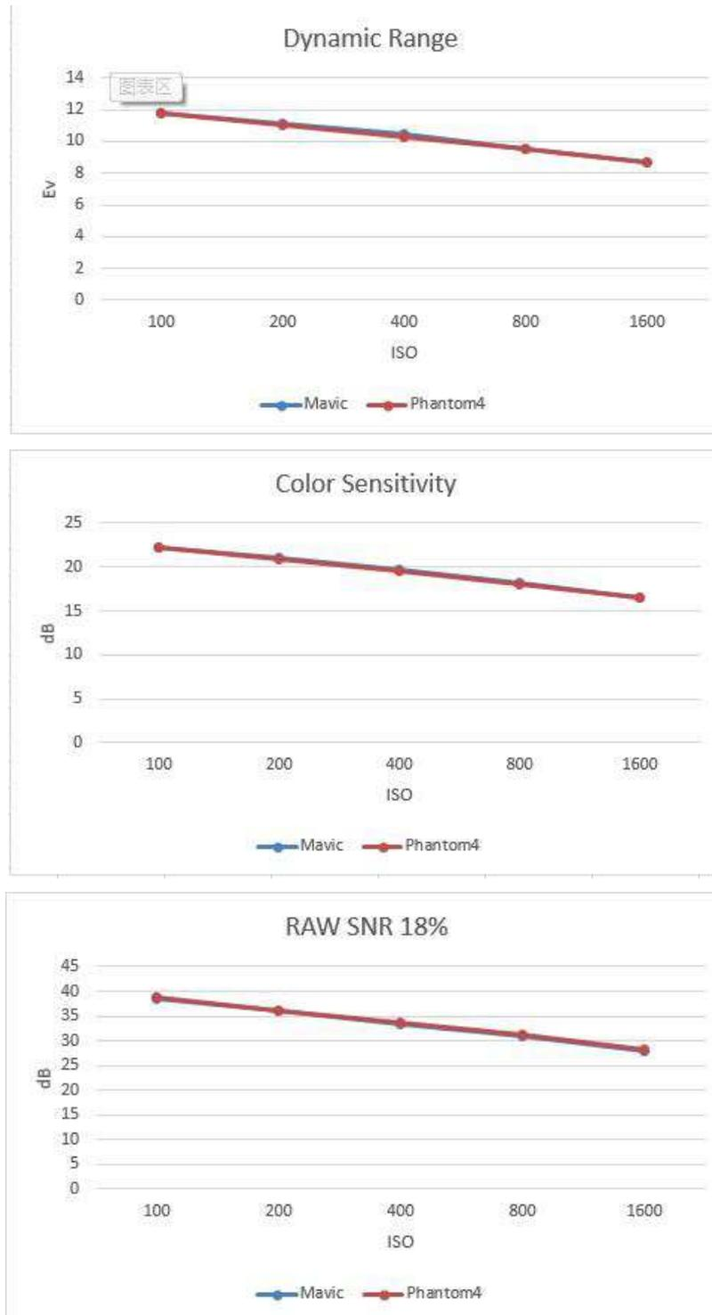
Figure 1 Comparisons of the dynamic range, color sensitivity and SNR 18% of Mavic Pro and Phantom 4
